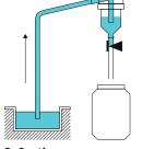
Suction: the air pump creates a vacuum in the sample chamber. The medium is sucked up through the suction hose until it reaches the level pen again.
